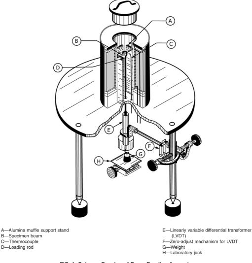
FIG. 1 Cutaway Drawing of Beam-Bending Apparatus
